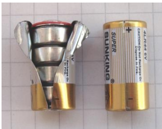
A partially opened 4LR44 battery showing the arrangement of the 4 1.5V LR44 cells; with an intact example for comparison
