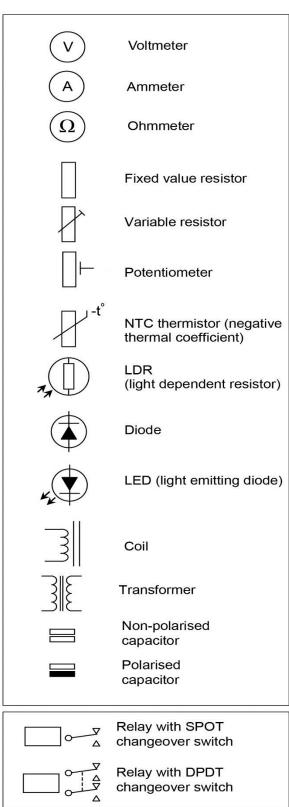
Identify the component symbols and use the following names to label 14 components:
